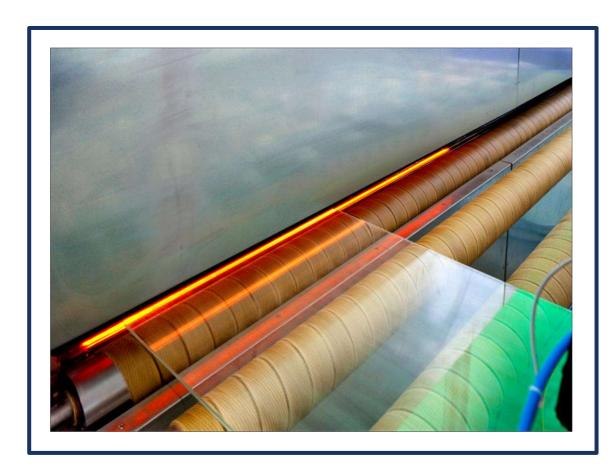
Tempered glass is a type of safety glass processed by heat or chemical treatments, to increase its resistance compared to normal glass. This is accomplished by putting the outer surfaces in compression and the inner surfaces in tension. These stresses mean that when glass is broken it crumbles into small pieces instead of breaking into large fragments.
